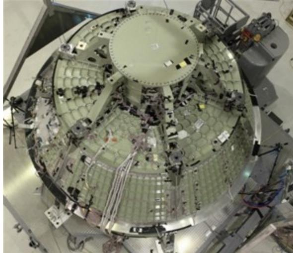
Figure 2. Orion Crew Module During Proof Pressure Test (Photo Courtesy of Lockheed Martin Space Systems)
