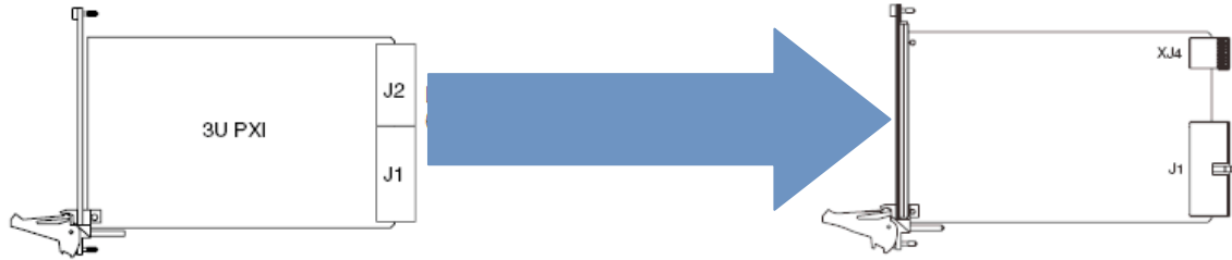
Figure 3. Hybrid-slot-compatible PXI modules include the smaller XJ4 connector in place of the larger J2 connector.
