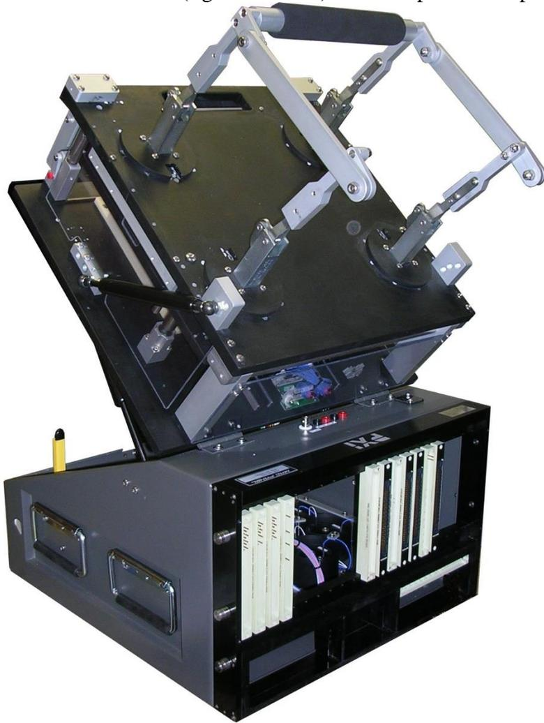
(Fig 5: Functional fixture with a manual top drive unit. This fixture accesses the DUT using a ramp driven side access unit which means that as the top is engaged by the operator the side access is automatically driven into the connector of the DUT. Image courtesy of Circuit Check Inc.)
