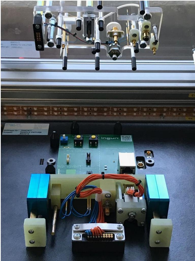
(Figure 4: Bed of Nails Test Fixture. Photo Courtesy of iBtest)
