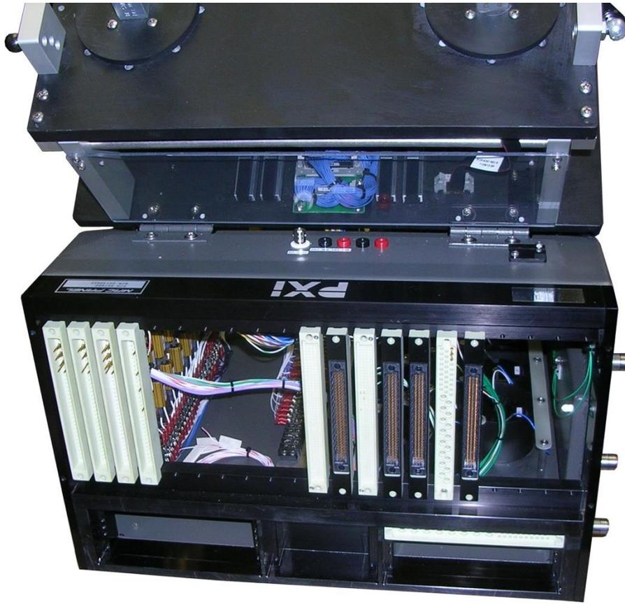
(Fig 6: Same functional fixture as above. You can see the cabling from the fixture plate down to the mating modules. The mating modules are mounted onto a MAC Panel SCOUT ITA which then mounts onto a SCOUT Receiver with mating DAKs (direct access kit) mass interconnect technology. Image courtesy of Circuit Check Inc.)
