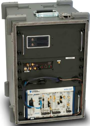
Figure 3 – RF Shielded Box Protects against Interference
